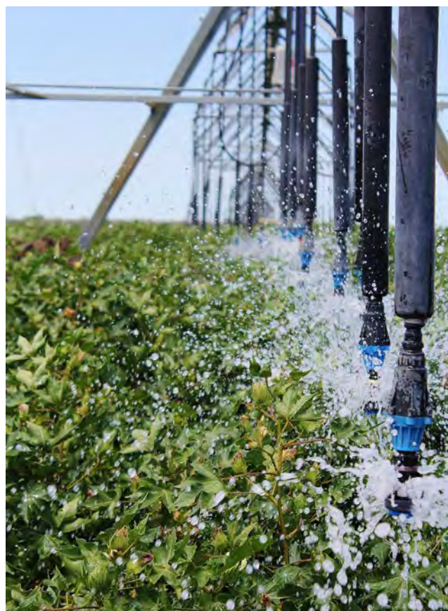
Overhead irrigation, such as centre pivots or laterals, has higher establishment costs but potential for improved yield and water use efficiency.
