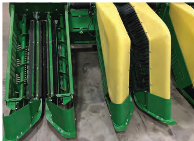
The stripper uses brushes and bats to strip seed cotton from bolls. © René van der Sluijs
