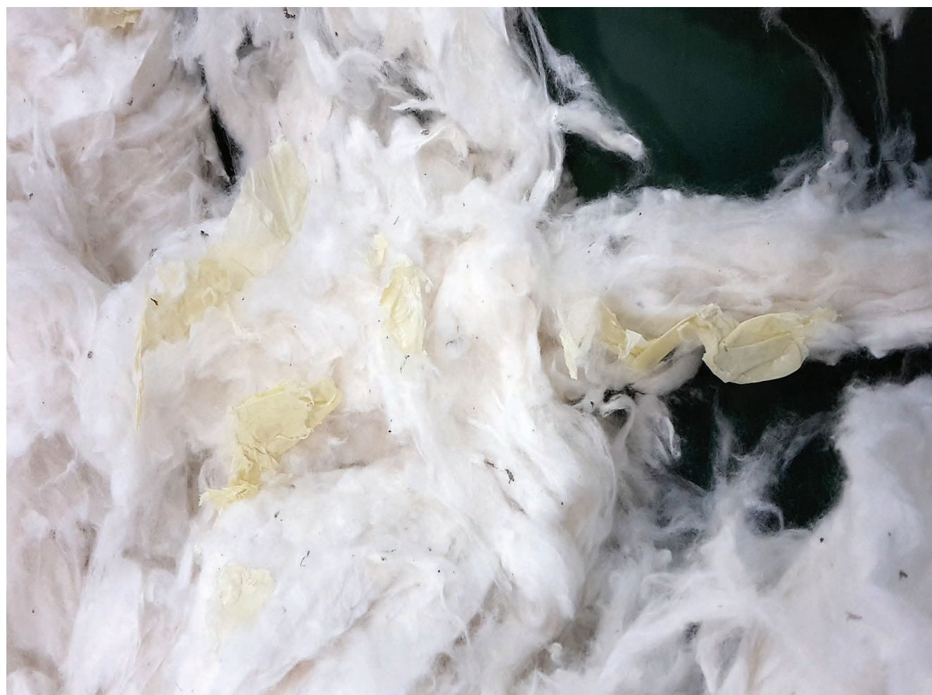
Round module plastic wrap in cotton bale. © René van der Sluijs
