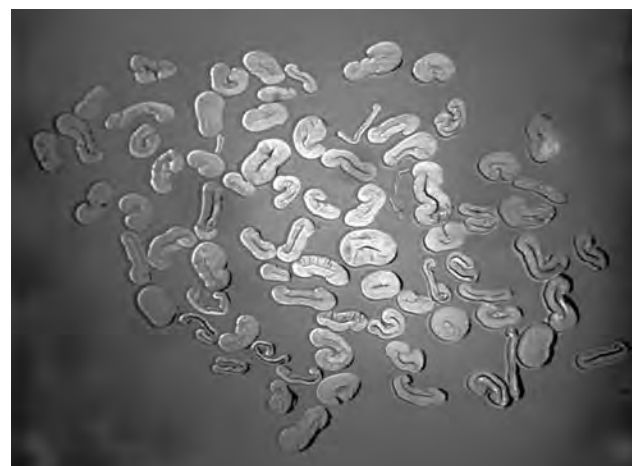
Cross-section of a cotton yarn showing the packing and interaction of individual fibres. Changes in micronaire affect how many fibres make up the cross section of the yarn, impacting its strength and dye uptake. © CSIRO
